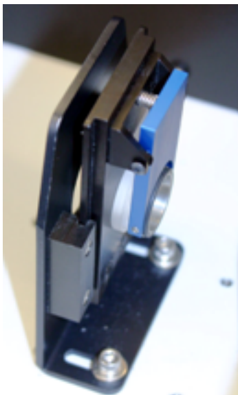
Figure 2: Close-up of the salt plates in the IR instrument, ready to take a sample
