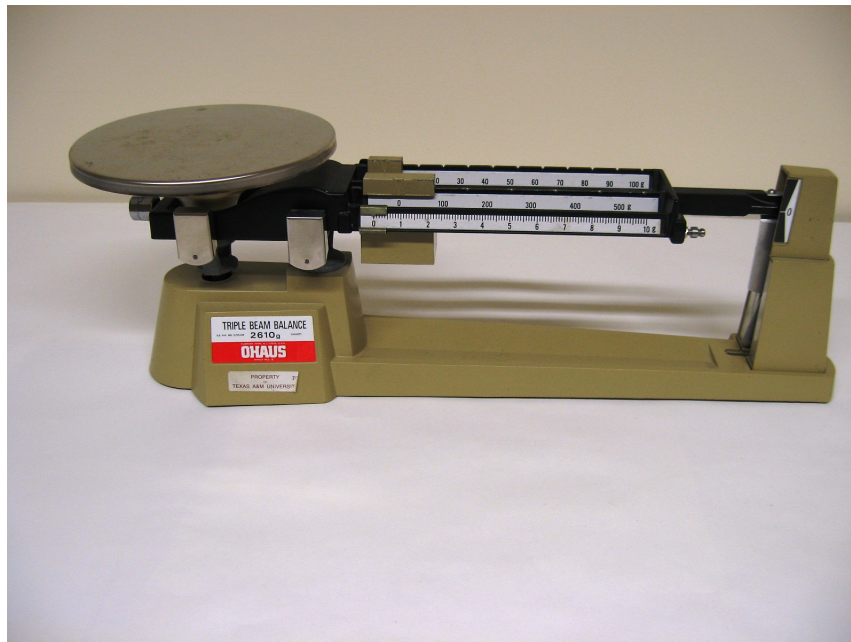
Figure 2: Triple beam balance
