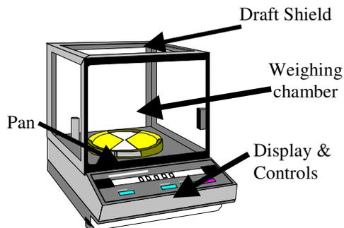
Analytical balances are used for very accurate, quantitative measurements of mass to the nearest 0.001 g. (Some read to 0.0001 g.) They are delicate instruments, subject to errors caused by vibration and drafts. These problems can be minimized with care and a certain amount of common sense.
