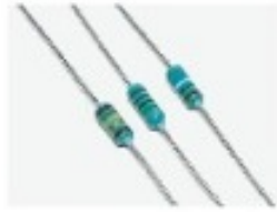
Figure 2: Color-coded ceramic resistors
