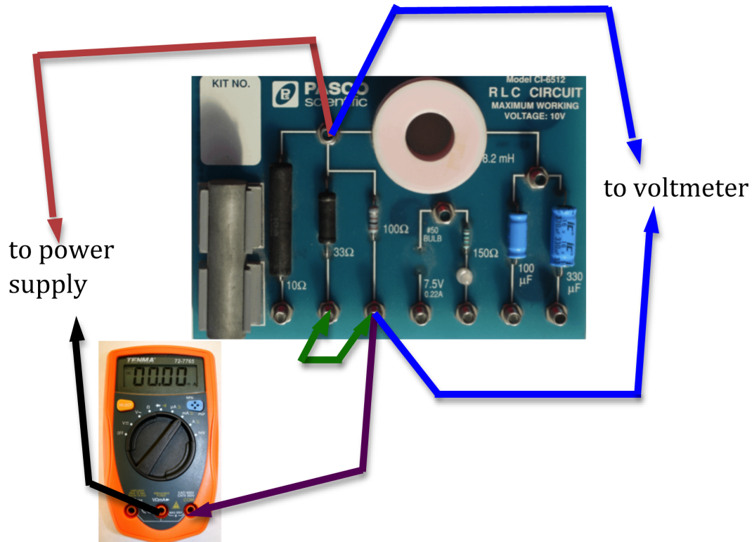
Figure 11: Connection for parallel circuit
