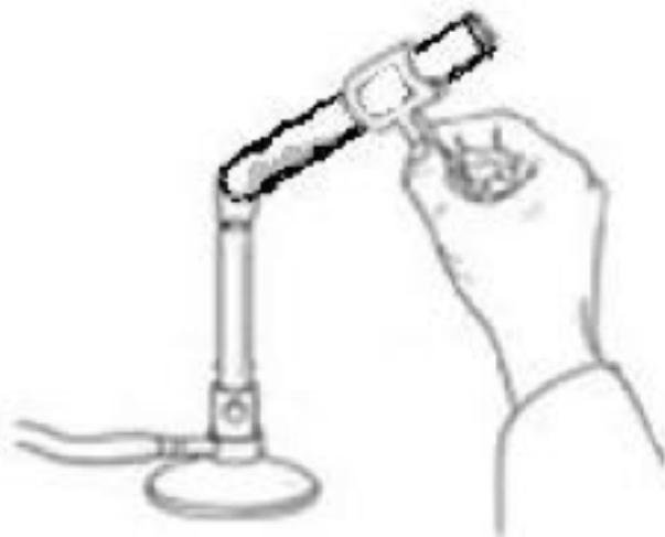
Figure 1: How to evaporate water from a hydrate.
