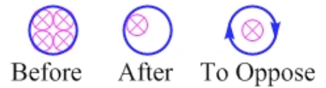
Figure 20.29: The pictorial method applied to the region that is leaving the magnetic field.
