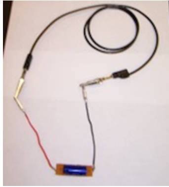
Figure 5: Discharging a capacitor
