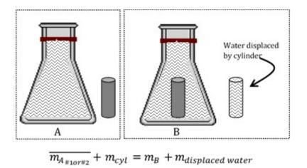
Calculate the volume of the metal cylinder and its uncertainty based on your mass measurements.
