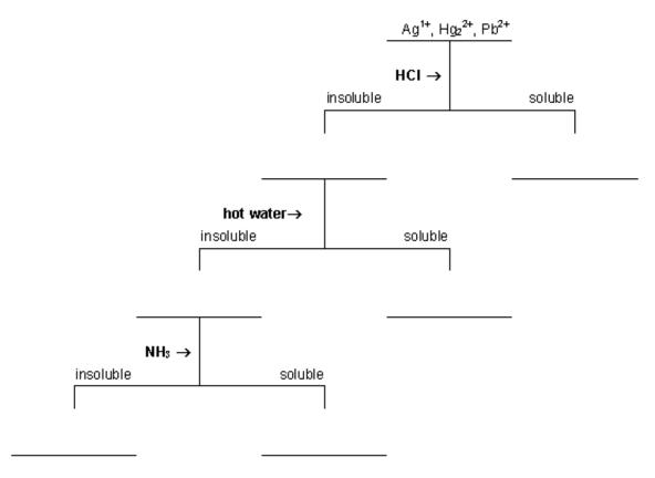
Figure 1: Flow Chart for Separation of Mixture of Ag<sup>+</sup>, Hg<sub>2</sub> <sup>2+</sup>, Pb<sup>2+</sup>. Each "soluble" branch should be tested with KI to confirm the presence of an ion.
